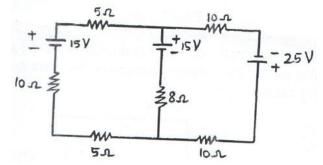
12 For the circuit shown below calculate impedance, current, voltage across in each element, active power, reactive power and power factor. Also draw the phasor diagram. (10)
