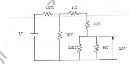
b) Using the Thevenin's theorem determine Vo in circuit below
