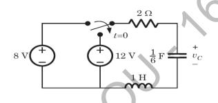
(b) The capacitor voltage and inductor current at t = 0<sup>-</sup> (just before the switch is closed)
