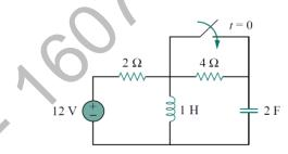
14 (a) Find V<sub>0</sub>(t) in the given circuit below, V<sub>0</sub>(O) = 5V by using Laplace transform
