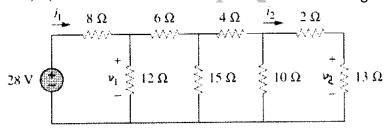
b) Write procedure for solving circuit using superposition theorem and calculate current through 4 resistor in the circuit shown below by superposition equivalent.
