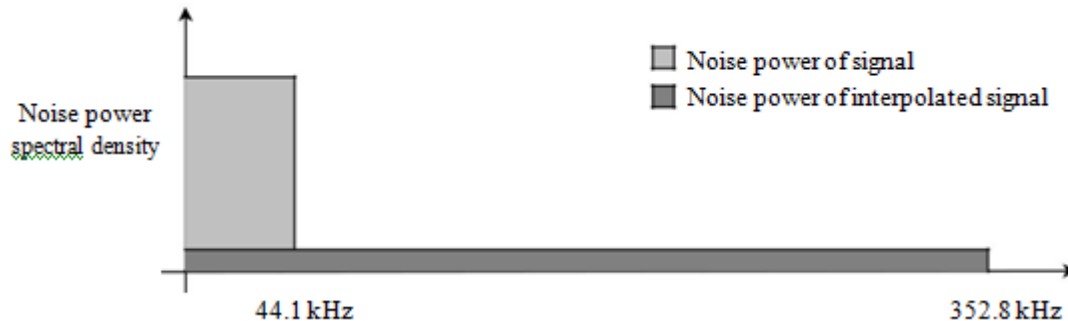
Figure 5.11: Illustration of noise power spectral density reduction due to oversampling.
