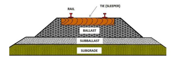
**GAUGE** The clear minimum horizontal distance between the inner (running) faces of the two rails forming a track is known as Gauge. Indian railway followed this practice. In European countries, the gauge is measured between the inner faces of two rails at a point 14 mm below the top of the rail.
