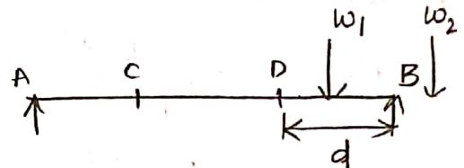
$$\text{at } x = L-d \quad M_{x_1} = \frac{w_1 d (L-d)}{L}$$
