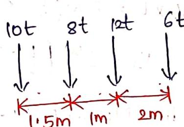
Distance between chosen load and  $\Sigma w$  is
