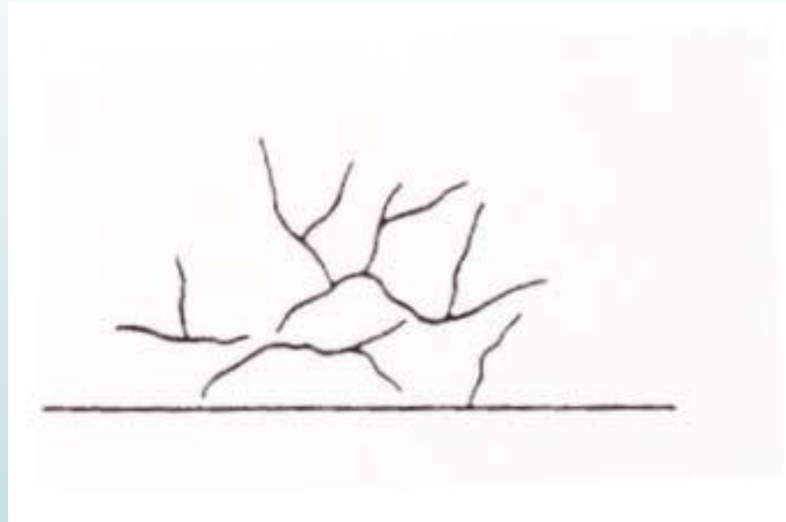
Fig. 1. Sketch of surface appearance when concrete has been mixed for too long or the time of transport has been too long.
