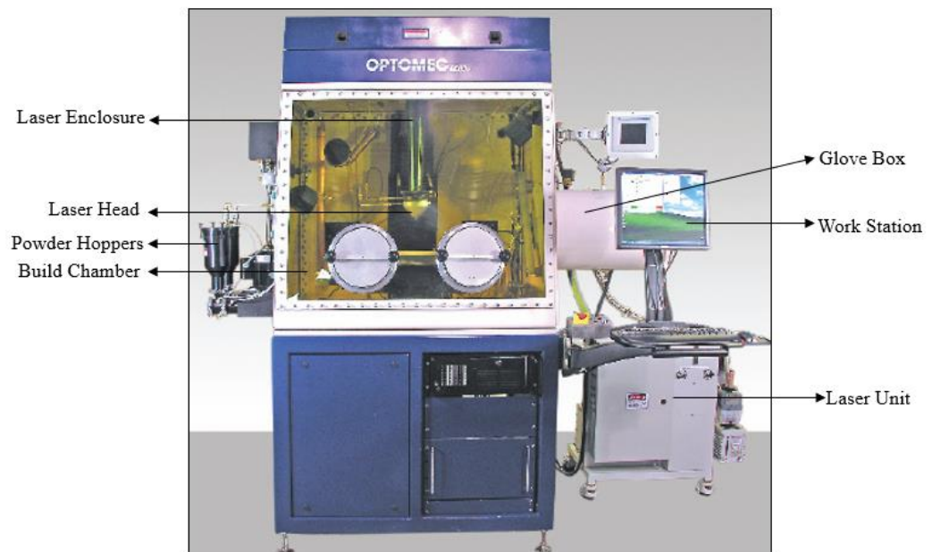
Figure3.2: LENS machine setup
