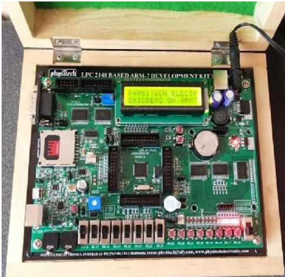
Fig. 1: Physitech LPC-2148 BASED ARM-7 DEVELOPMENT KIT
