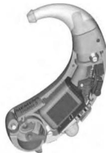
Fig. 1.3 A digital hearing aid employing signal processing technique
