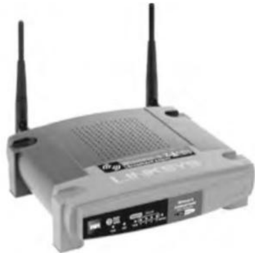
Fig. 1.2 A wireless network router for data communication (Photo courtesy of Linksys (www.linksys.com). A division of CISCO system)
