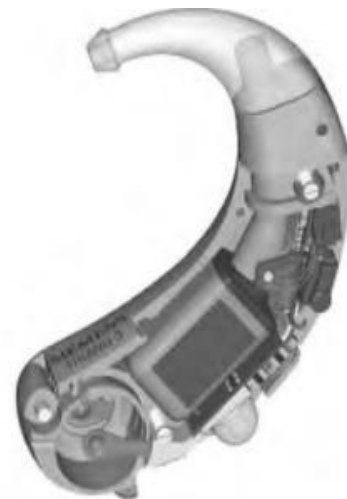
Fig. 1.3 A digital hearing aid employing signal processing technique (Siemens TRIANO 3 Digital hearing aid; Siemens Audiology Copyright© 2005)
