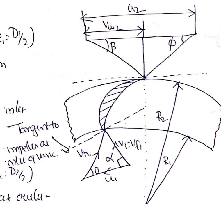
$V_{w2}, V_h, V_p, \beta$  and  $\phi$  are the corresponding values at outlet while passing through the impeller. The velocity of which changes and there is a change of moment of momentum.
