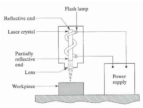
**Laser Tube & Lamp Assembly** (main part). The following parts are fitted inside an enclosure, which carries good quality reflecting surfaces inside.
