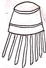
TO-5 Style Package with straight leads
