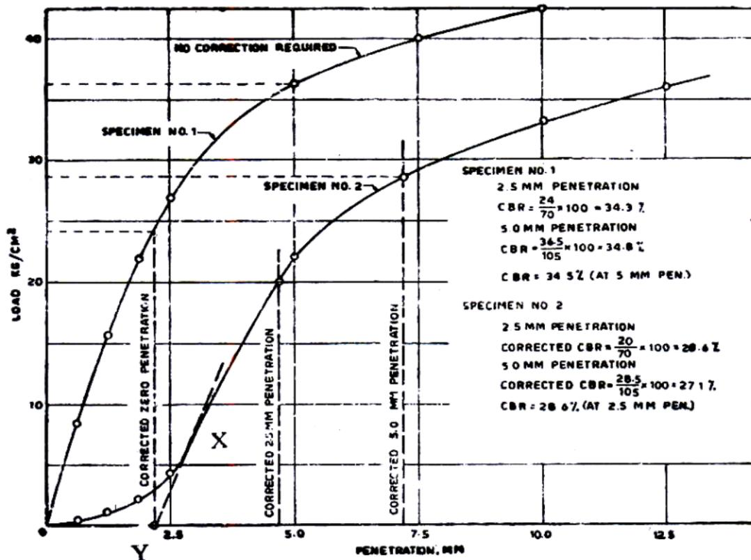
C.B.R. Test Load-Penetration Curve
