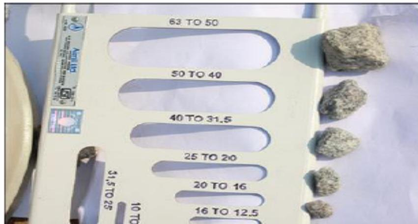
**Aggregate passed along the thickness**
