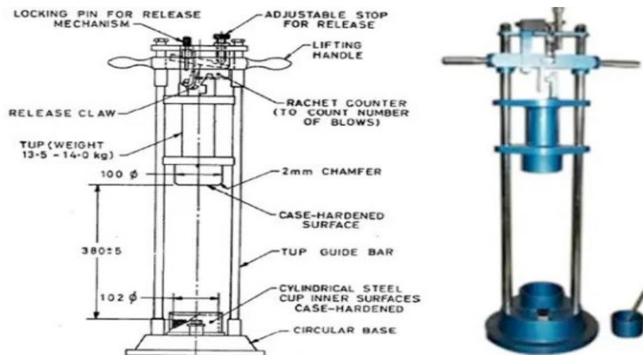
**Aggregate Impact Test Apparatus**
