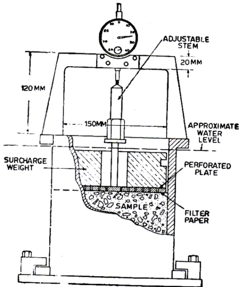
**C.B.R. Mould with Swell Measuring Device**
