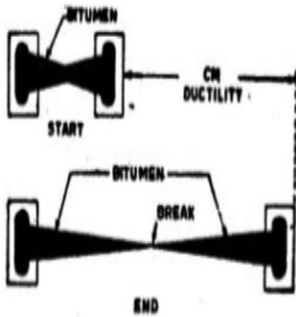
Figure 18.1 Ductility Test Concept
