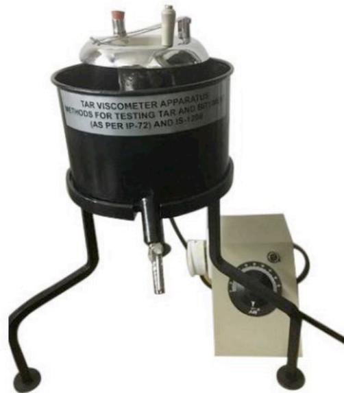
Tar Viscometer apparatus
