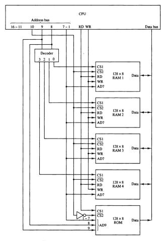
Figure 12-4 Memory connection to the CPU.
