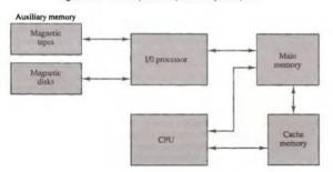
Figure 12-1 Memory hierarchy in a computer system.
