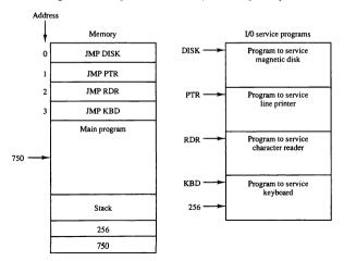
Figure 11-15 Programs stored in memory for servicing interrupts.
