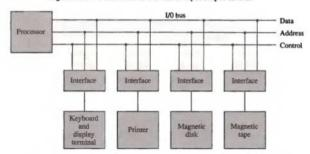
Figure 11-1 Connection of I/O bus to input-output devices.
