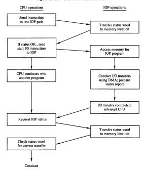
Figure 11-20 CPU-IOP communication.
