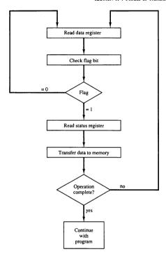
Figure 11-11 Flowchart for CPU program to input data.
