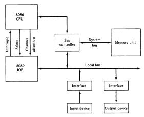
Figure 11-23 Intel 8086/8089 microcomputer system block diagram.
