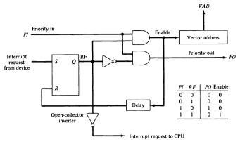
Figure 11-13 One stage of the daisy-chain priority arrangement.
