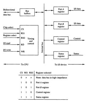
Figure 11-2 Example of I/O interface unit.
