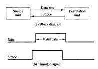
Figure 11-4 Destination-initiated strobe for data transfer.
