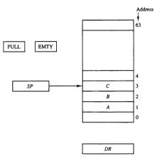
Figure 8-3 Block diagram of a 64-word stack.
