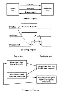
Figure 11-5 Source-initiated transfer using handshaking.
