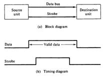
Figure 11-3 Source-initiated strobe for data transfer.
