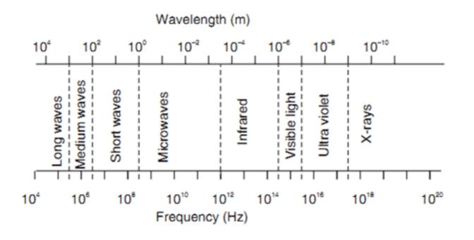
Among these waves microwaves, infrared waves and visible light waves are useful for the distance measurement.
