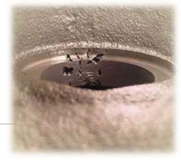
Porosity is in the form of cavities caused due to gas entrapment during solidification.
