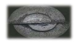
The casting that does not match at the parting line is known as Mismatch or Mould shift.
