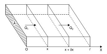
The amount of heat crossing any section of the bar per second depends on the area A of the cross-section, the conductivity K of the material of the bar and the temperature gradient  $-\frac{u}{x}$  *i.e.*, rate of change of temperature w.r.t. distance normal to the area.
