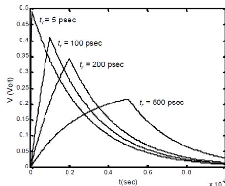
**CAPACITIVE COUPLING TO A DRIVEN LINE AND ITS VOLTAGE RESPONSE**
