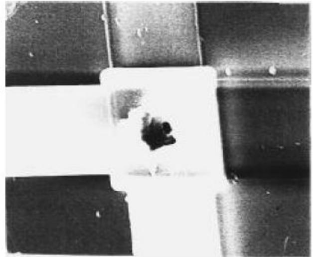
*Open Failure in Contact Plug***ELECTROMIGRATION RELATED FAILURE MODES**
