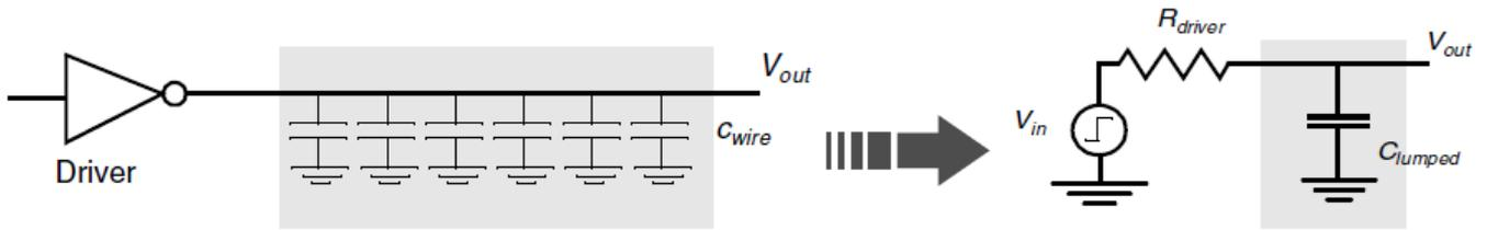
**DISTRIBUTED VERSUS LUMPED CAPACITANCE MODEL OF WIRE.**  $C_{LUMPED} = L \times C_{WIRE}$ , WITH  $L$  THE LENGTH OF THE WIRE AND  $C_{WIRE}$  THE CAPACITANCE PER UNIT LENGTH. THE DRIVER IS MODELED AS A VOLTAGE SOURCE AND A SOURCE RESISTANCE  $R_{DRIVER}$
