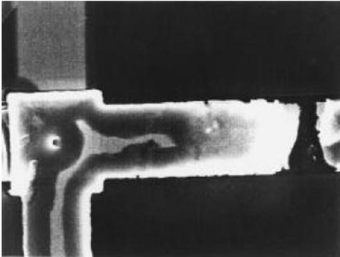
*Line Open Failure*
