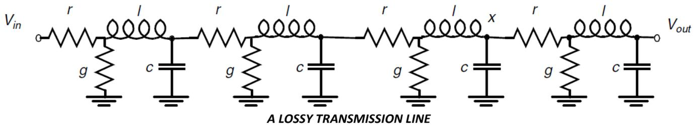
Consider the point  $x$  along the transmission line of figure as shown above at time  $t$ . The following set of equations holds:
