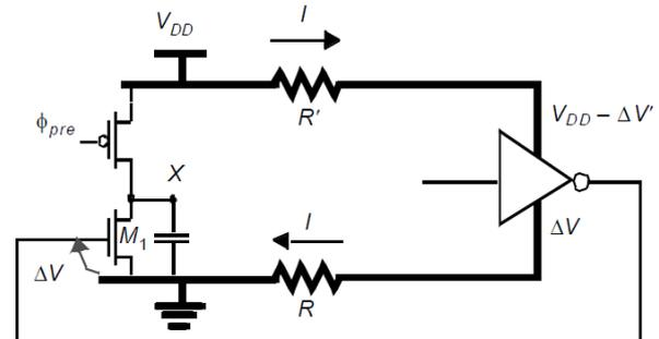
OHMIC VOLTAGE DROP ON THE SUPPLY REDUCES NOISE MARGIN
