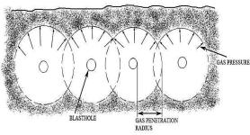
Fig. 2. Gas Pressure Applied Load at the Periphery of Hydrostatically Stressed Cylinders Causing Rock Movement. [7]
