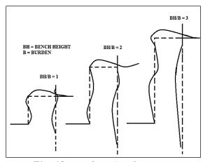
Fig. 12. Bending Conditions in Blasting. [32]
