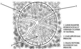
*Fig. 1.* Hydrostatic Stress Field Created Around a Blast hole. [6]
