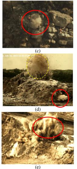
Fig. 13. Escape of Gas Energy Through Weak Planes and Stemming Zone.
