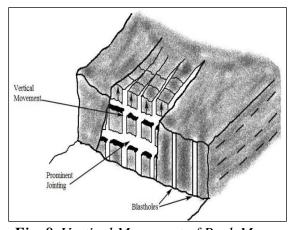
Fig. 8. Vertical Movement of Rock Mass.
