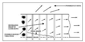
**Fig. 10.** Effect of Insufficient Burden Relief.
