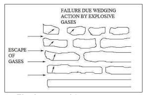
Fig. 4. Escape of Gases into Joints.
