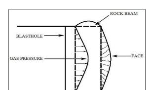
**Fig. 3.** Rock Breaking by Flexural Bending. [8]
