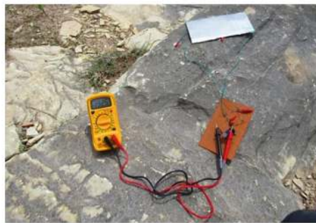
Fig. 2. Extraction of electricity using Piezo-Gen circuit from undesirable blast vibrations at limestone mine
