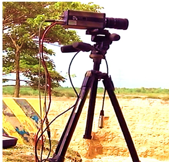
Figure 2. High speed video camera of 1000fps capacity
