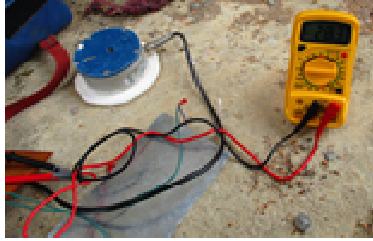
Fig. 2(b). Extraction of electricity using piezo-gen circuit from undesirable blast vibrations.
