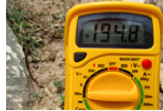
Fig. 2(c). Observation of obtained voltage from the blast vibrations undesirable by multimeter for the assessment of seismic energy.
