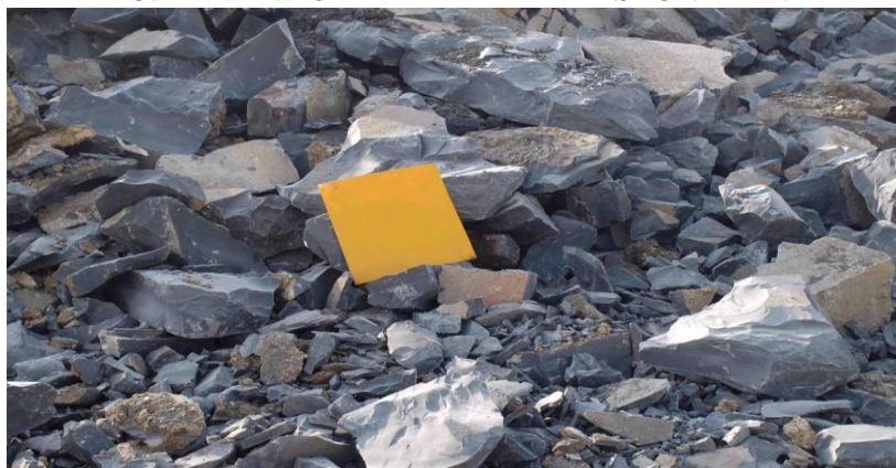
FIG. 13 CALIBRATOR FOR FRAGMENTATION ASSESSMENT USING WIPFRAG TABLE - 4 JOINT SPACING AND FRAGMENTATION INFORMATION FOR BLASTS
