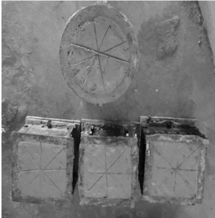
Fig. 1 Casting of Geopolymer specimens
