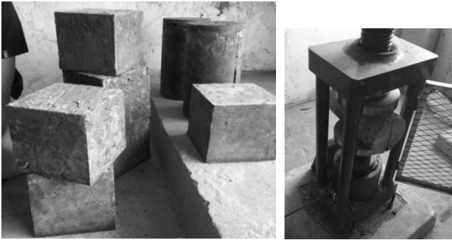
Fig. 2 Demoulded concrete specimens
