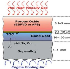
Figure 3. Different layers of coating and their thicknesses
