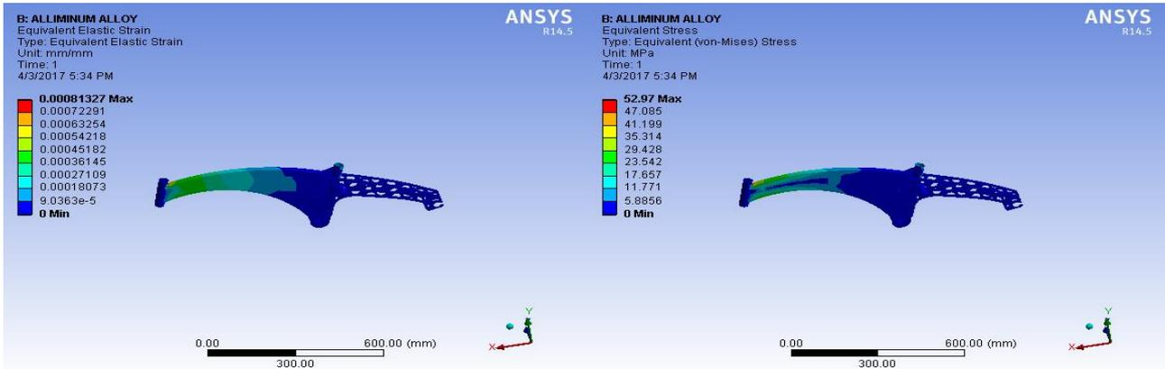
Fig: 8 Equivalent elastic strain and Vonnises Stress
