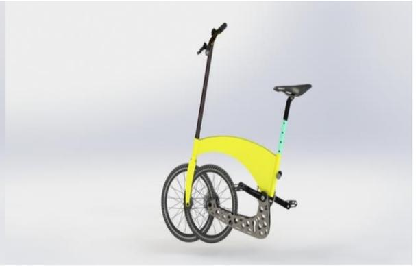
Fig :5 Folded view of the cycle
