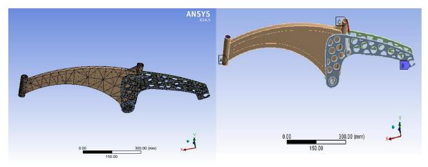
Fig:7 Meshing and Boundary conditions applied to the frame
