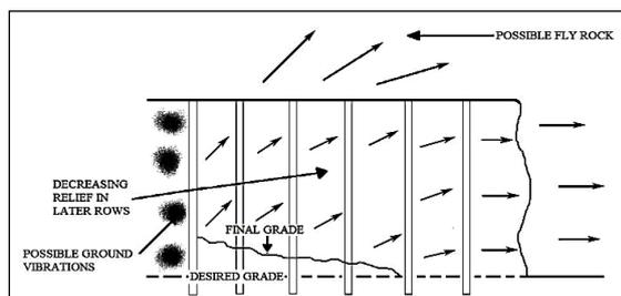
Fig. 10. Effect of Insufficient Burden Relief.
