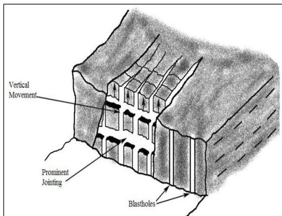
**Fig. 8.** Vertical Movement of Rock Mass.
