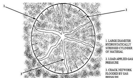
**Fig. 1.** Hydrostatic Stress Field Created Around a Blast hole.<sup>[6]</sup>
