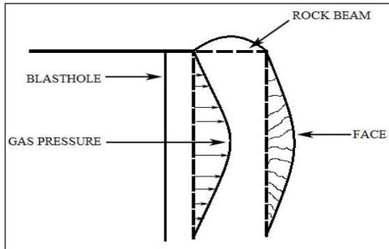
Fig. 3. Rock Breaking by Flexural Bending.<sup>[8]</sup>
