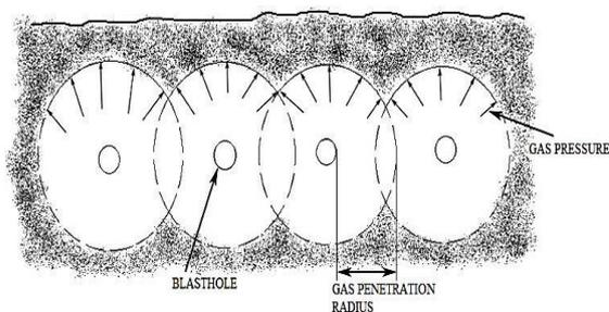
**Fig. 2.** Gas Pressure Applied Load at the Periphery of Hydrostatically Stressed Cylinders Causing Rock Movement.<sup>[7]</sup>
