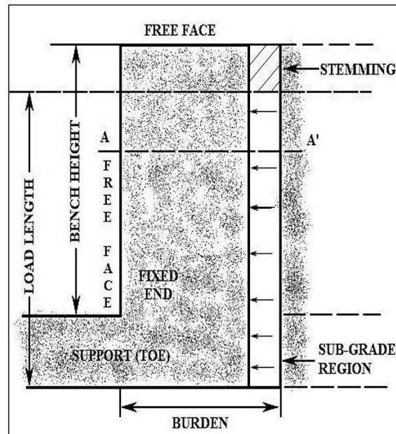
Fig. 11. Analogy Between Burden Rock and a Structural Beam.<sup>[8]</sup>
