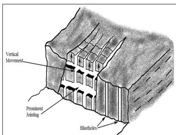
**Fig. 8.** Vertical Movement of Rock Mass.
