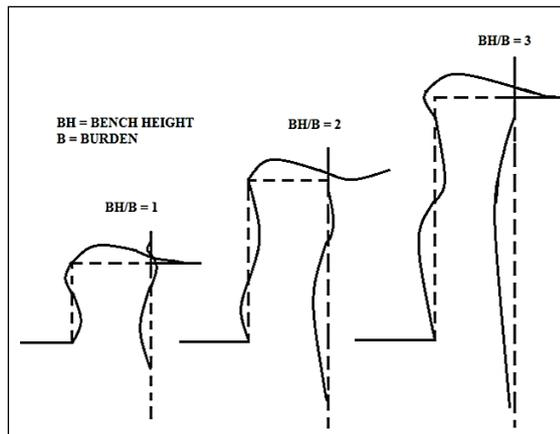
Fig. 12. Bending Conditions in Blasting.<sup>[32]</sup>
