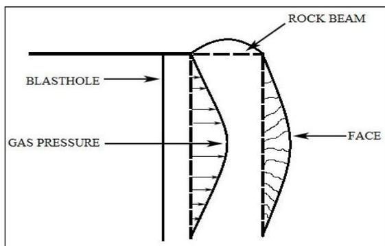
Fig. 3. Rock Breaking by Flexural Bending.<sup>[8]</sup>
