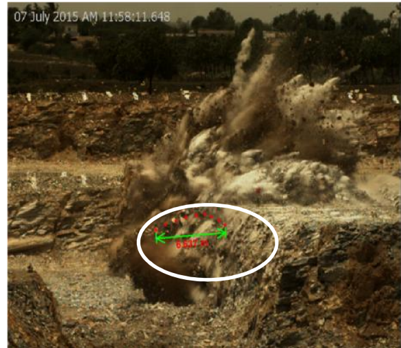
Displacement of rock movement obtained as 6.637m
