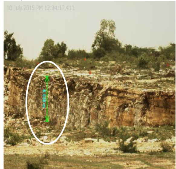
Height of the bench obtained as 8.538m
