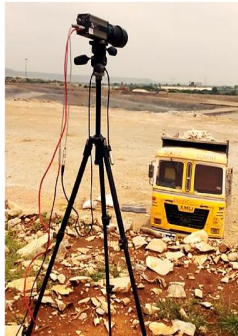
Figure 2: High speed video camera of 1000fps capacity
