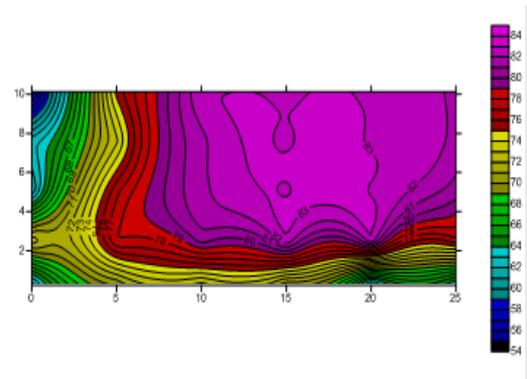
**Figure 10** Transverse Velocity Contours of Sec 3 by Numerical Analysis **Figure 11** Transverse Velocity Contours of Sec 3 from Experiment
