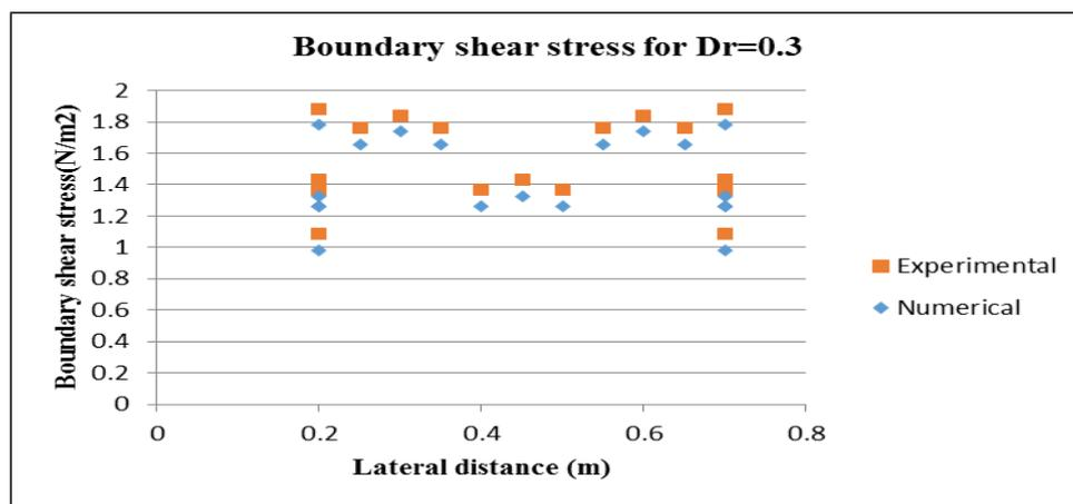
Figure 14 Boundary shear stress of Sec 3
