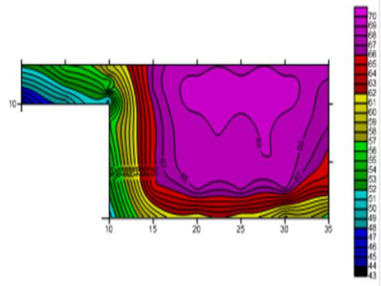
**Figure 8** Transverse Velocity Contour of Sec 2 by Numerical Analysis **Figure 9** Transverse Velocity Contour of Sec 2 from Experiment
