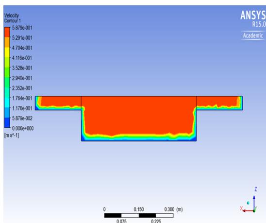
**Figure 6** Transverse Velocity Contour of Sec 1 **Figure 7** Transverse Velocity Contour of Sec 1 by Numerical Analysis
