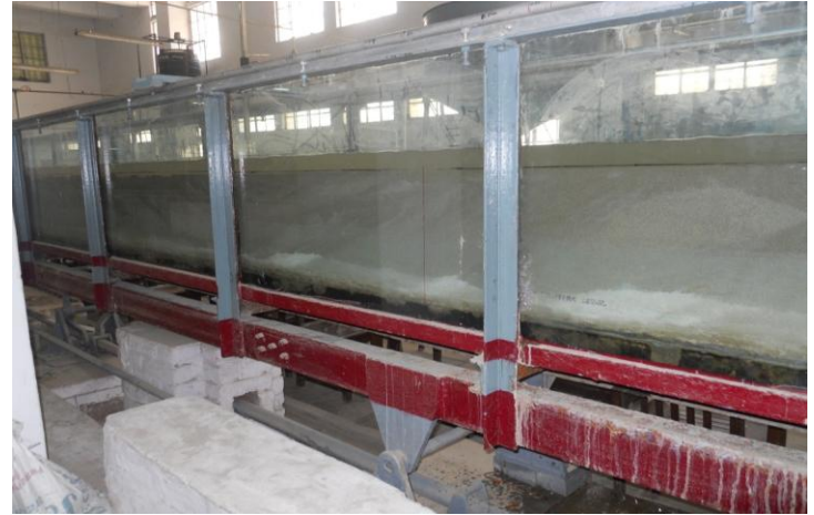
Figure 1. A view of the experimental flume.
