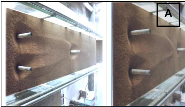
Figure- 2. Scour and deposition patterns around piers placed in staggered arrangement at varied pier spacing (A) X_c/b=50 (B) X_c/b=60
