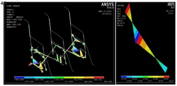
Figure 10: Bending Moment at various positions
