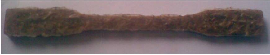
Fig. 17.1 Coir fiber-reinforced polyester composite tensile test specimen
