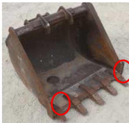
Figure 2: Failure in tooth due to impact loading and abrasion wear
