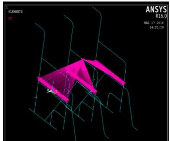
Figure 7: Mass Element Coupled With The chassis
