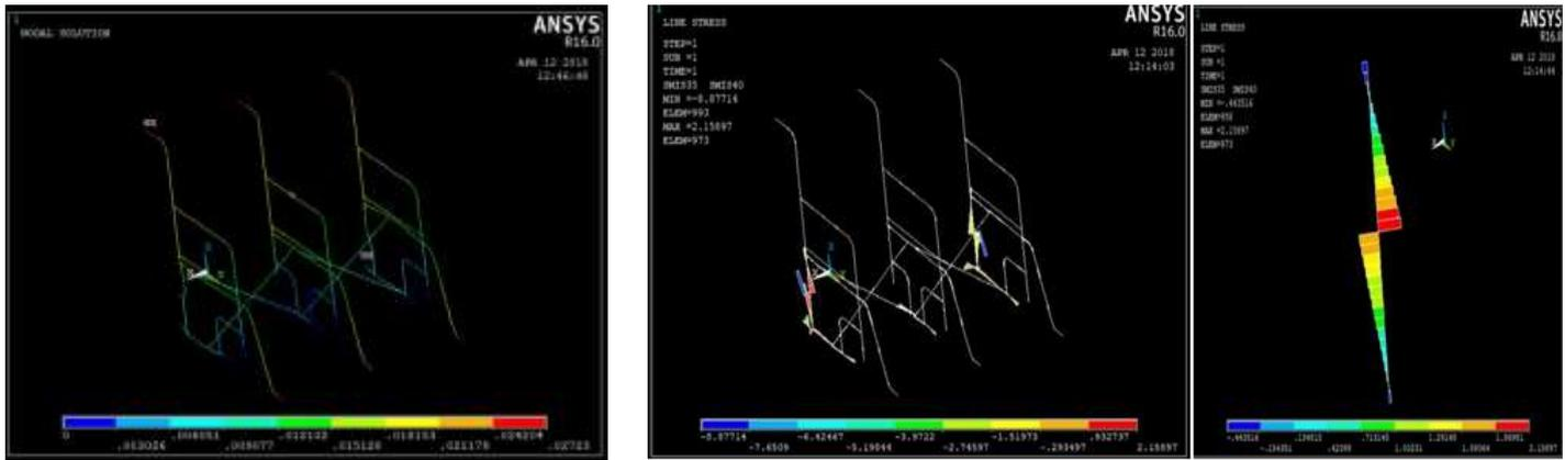
Figure 8: Deformation of the Model Figure 9: Bending Stresses Developed at various positions
