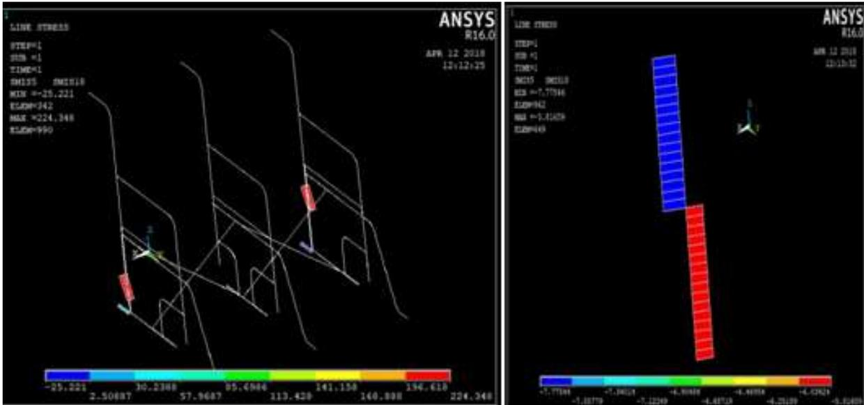
Figure 12: Shear Forces Developed at various positions
