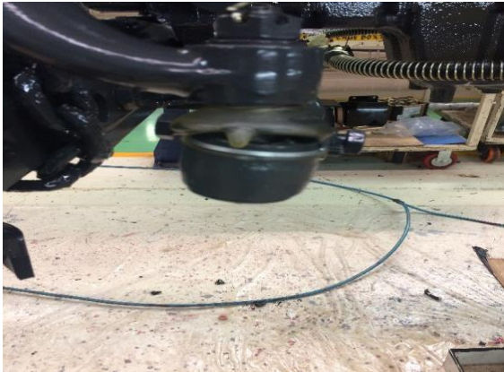
Fig 1.1: Damaged Rubber Boot
