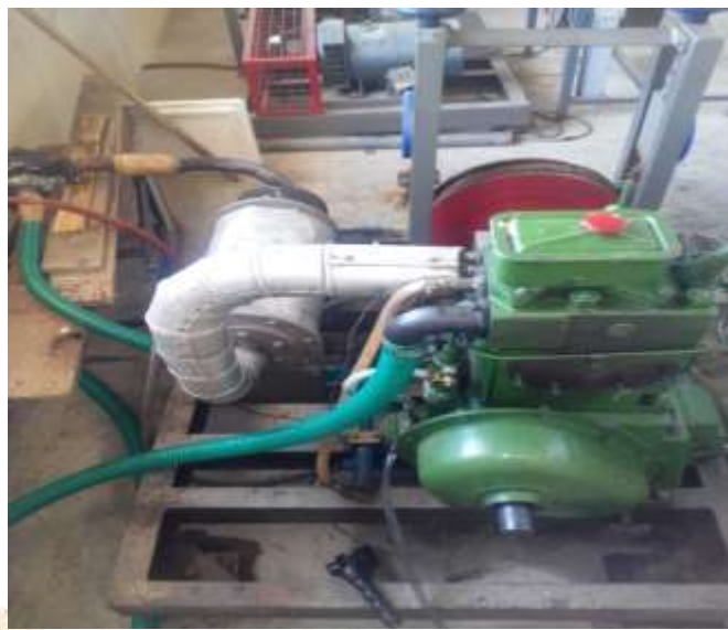
Figure 3: Modified Intake System (Intake from Turbo)
