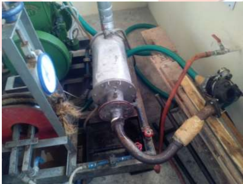
Figure 4: Modified Exhaust System (Exhaust to Turbo)
