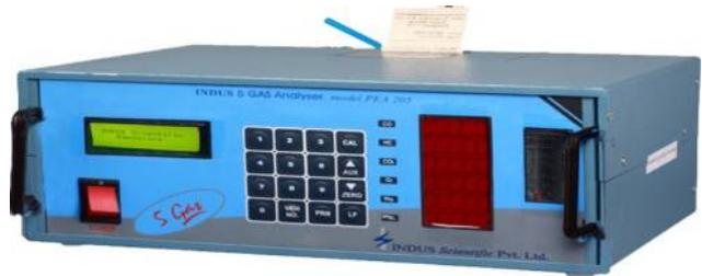
for monitoring five gases, namely, CO, CO<sub>2</sub>, HC, O<sub>2</sub> and NO<sub>x</sub> from the engine exhaust. It is made such that it meets the OIML Class I specifications. CO, CO<sub>2</sub> and HC (Hydrocarbon residue) are measured by NDIR technology, and O<sub>2</sub> and NO<sub>x</sub> are measured by electrochemical sensors.
