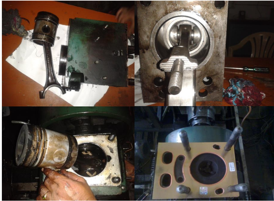
Fig. 4 Modified piston arrangement in cylinder
