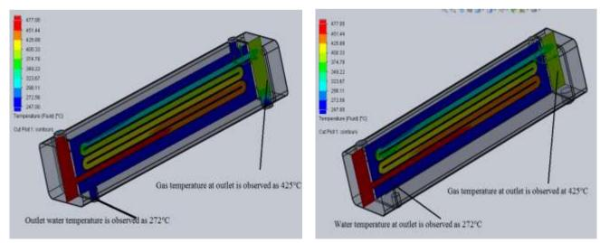
Figure 8. Temperature distribution across the 1st set of tubes Figure 9. Temperature distribution across the  $2^{nd}$  set of tubes for 25mm bends radius condition for 25mm bends radius condition
