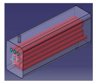
Figure 4. Isometric view of the assembly of the economizer for the CFD analysis Figure 5. Fluid model required
