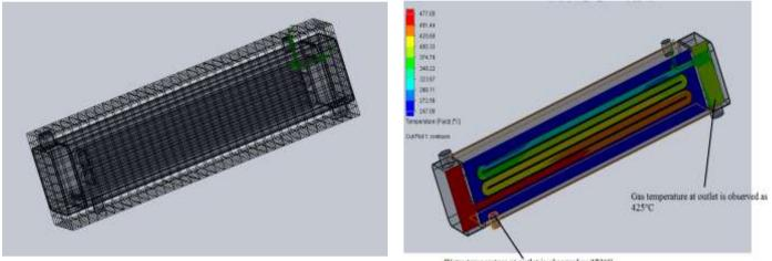
Water temperature at outlet is observed as 272°C
