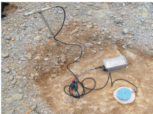
Figure 6. Monitoring of Ground Vibration
