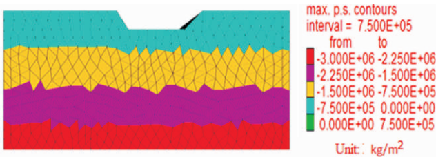
Figure 10. Distribution of Stress under Dynamic Loading
