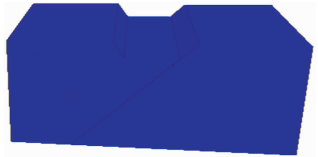
Figure 8. 3DEC Model of Canal Slope after Excavation
