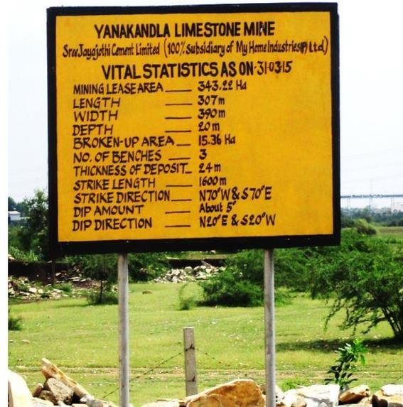
FIGURE II. STATISTICS OF YANAKANDLA LIMESTONE MINE AS ON 31.03.2015
