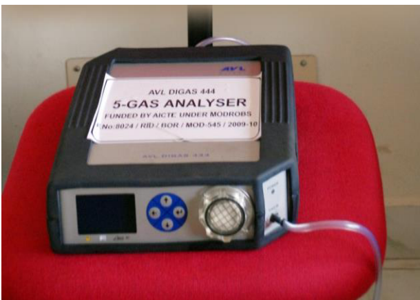
Figure 6. AVL Gas Analyzer
