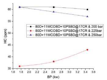
$Fig. 6. \ HC(ppm) \ v/s \ BP(kw) \ for \ a \ 20\% blended \ diesel \ from \ two \ different \ feedstock \ @ \ different \ injection \ pressure$
