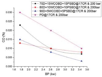
Fig. 2. CO % v/s BP(kw) for blends of biodiesel from two different feedstock and diesel @ 200bar injection pressure
