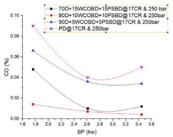
$Fig. 4.\ CO\ \%\ v/s\ BP(kw)\ for\ blends\ of\ biodiesel\ from\ two\ different\ feedstock\ and\ diesel\ @\ 250bar\ injection\ pressure$
