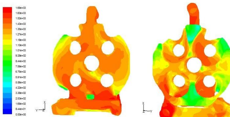
**Figure 12** Contour of Surface HTC Distribution ( $W/(m^2 \cdot K)$ )
