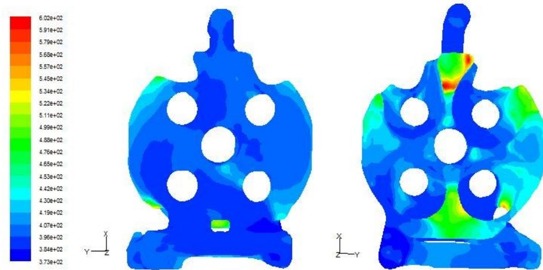
**Figure 13** Contour of Temperature Distribution at Wall (K)
