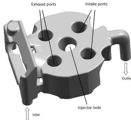
**Figure 2** Geometric Model of Cylinder Head Water Jacket
