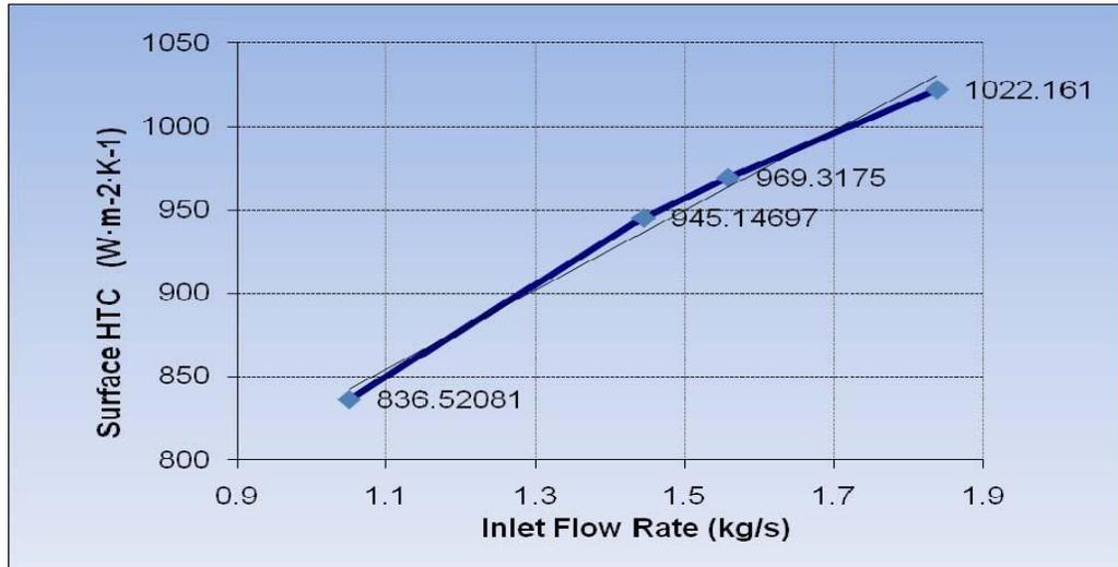
**Figure 19** Surface HTC at Different Flow Rates
