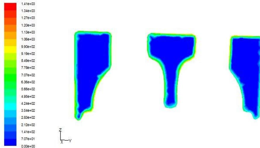
**Figure 10** Surface HTC ( $W/(m^2 \cdot K)$ ) on Nose Zones at  $x = -30$  mm
