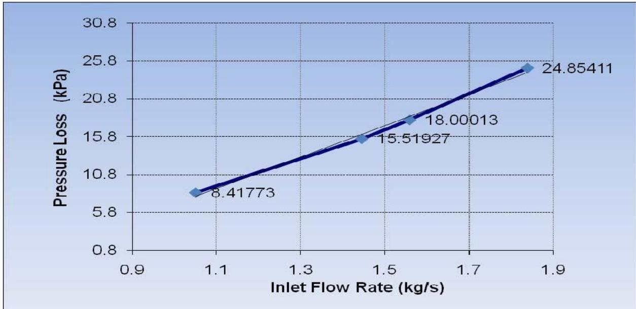
**Figure 17** Pressure Losses at Different Flow Rates
