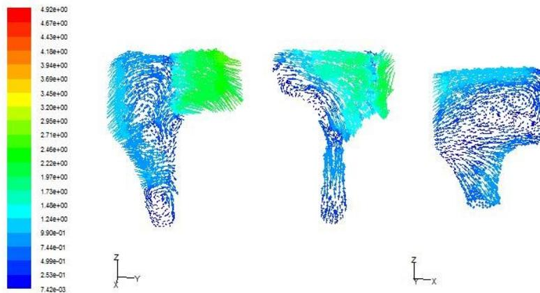
The higher flow rate in the narrow bridges between intake and exhaust valves ensured the cooling effects in the most problematic regions.
