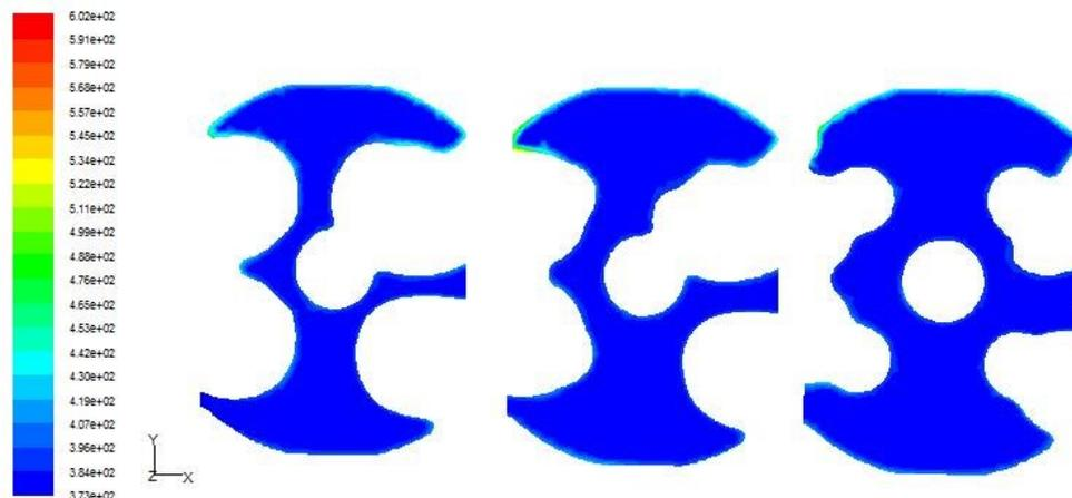
**Figure 14** Contour of Temperature Distribution at  $z = 35\text{mm}$ ,  $45\text{mm}$  and  $55\text{mm}$  (K)
