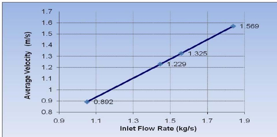
**Figure 18** Average Velocity at Different Flow Rates
