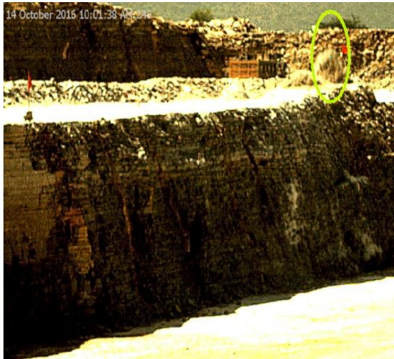
Escape of gas energy
