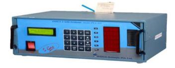
for monitoring five gases, namely, CO, CO<sub>2</sub>, HC, O<sub>2</sub> and NOx from the engine exhaust. It is made such that it meets the OIML Class I specifications. CO, CO<sub>2</sub> and HC (Hydrocarbon residue) are measured by NDIR technology, and O<sub>2</sub> and NOx are measured by electrochemical sensors.
