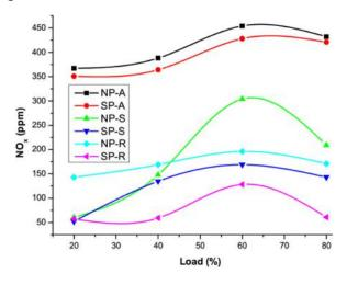
minimum  $NO_x$  emissions is 52 ppm at standard injection timing for the swirl piston at 20 per cent load and maximum 454 ppm is observed for normal piston with 60 per cent load at advanced injection timing.
